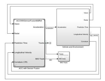
Figure 2: Adaptive cruise control schematic
